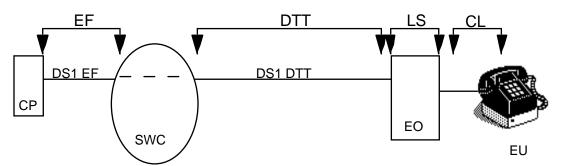
CP - Customer's Premises - Entrance Facility EF SWC - Serving Wire Center - Direct - Trunked Transport[1] DTT - Access Tandem ΑТ ΕO - End Office - Local Switching LS CL- Common Line
