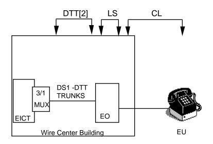
**EICT - DS3 Expanded Interconnection-Collocation Service Channel Termination**
